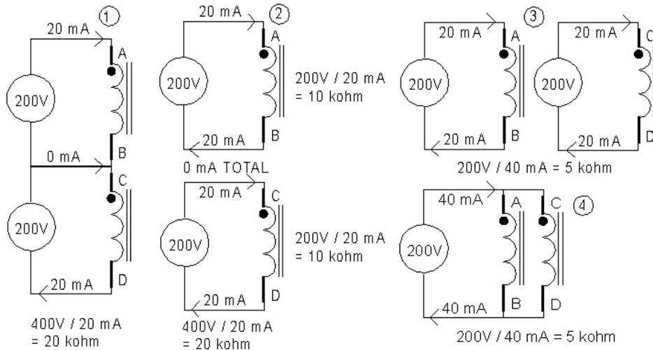
Starting with picture 1, we have a 400 V source consisting of two series 200V sources. This 400 V source is providing 20 mA into an effective load of 20 kohm. Notice that at the center tap (B C), there is zero total current flowing. The wire shown between the voltage source and the transformer does not have to be there.
